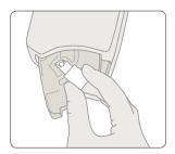
Place microcuvette into analyzer.
