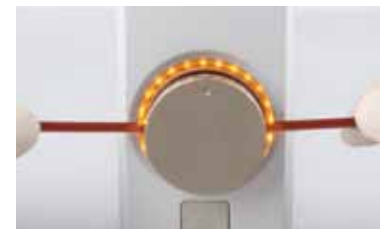
Sealing Sealing is complete in 0.5 to 3 seconds
