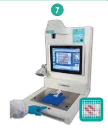
Press **SIZING** icon to superimpose a grid of 1 mm (or multiple thereof) to enable a precise sizing of the biopsies
