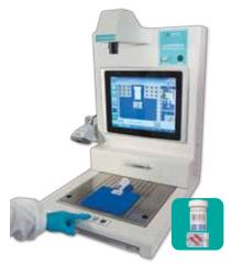
Transfer the specimen from the vial to the cassette. Place vial and cassette in the grooved bays on the blue colored cutting board. Press icon **CASSETTE/VIAL**
